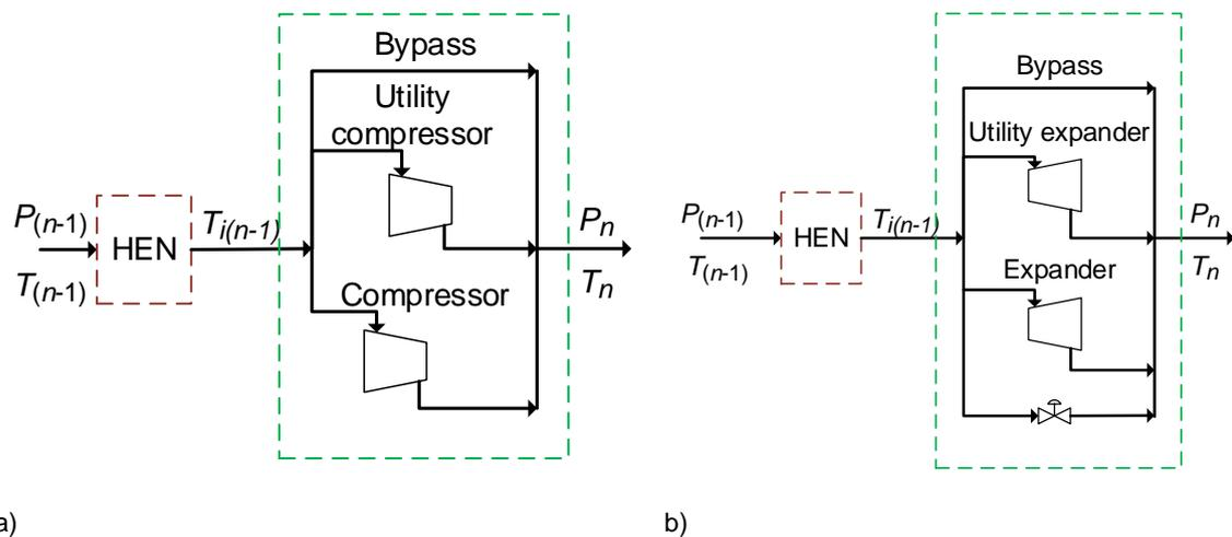
Figure 3: The WEN network at pressure stage  $n$  in the model by Huang and Karimi (2016): a) for low-pressure streams, b) for high-pressure streams
