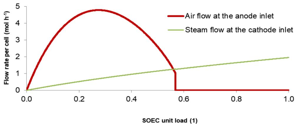
Figure 3: Inlet regulated air and steam flow rates as a function of the electrolyser unit power load
