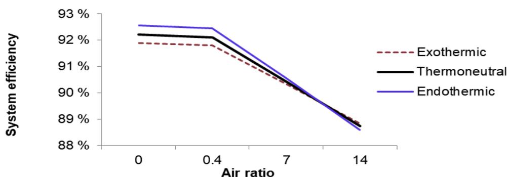
Figure 2: Impact of the air ratio (0; 0.4; 7; 14) on the system efficiency in three different modes
