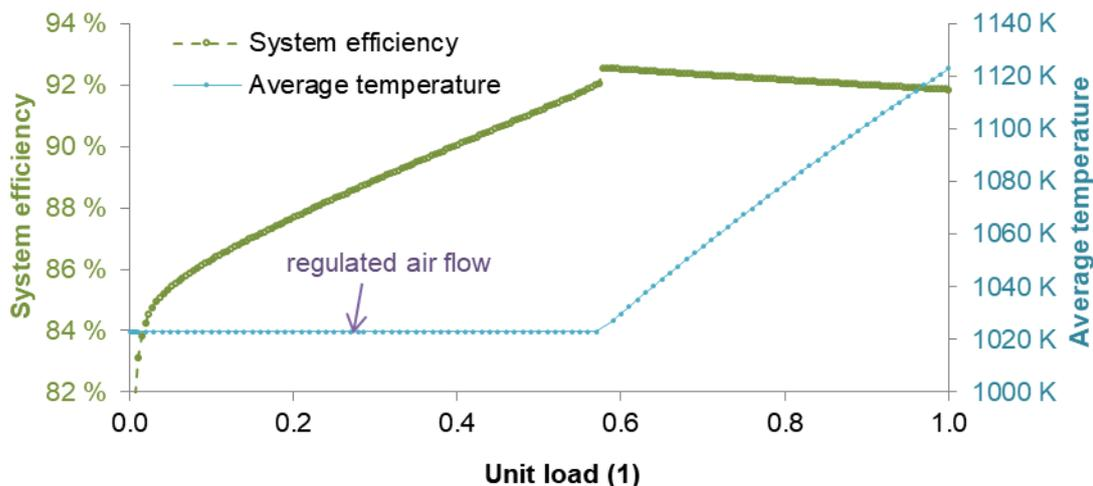
Figure 4: System efficiency and average temperature as a function of the system load in steady state, with a regulated air flow
