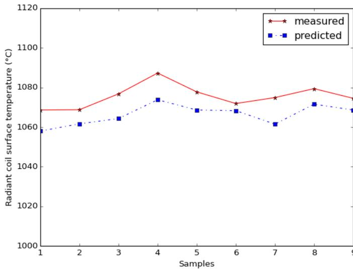
Figure 4: The coil surface temperatures of first group radiant coil in south side by measuring and predicting
