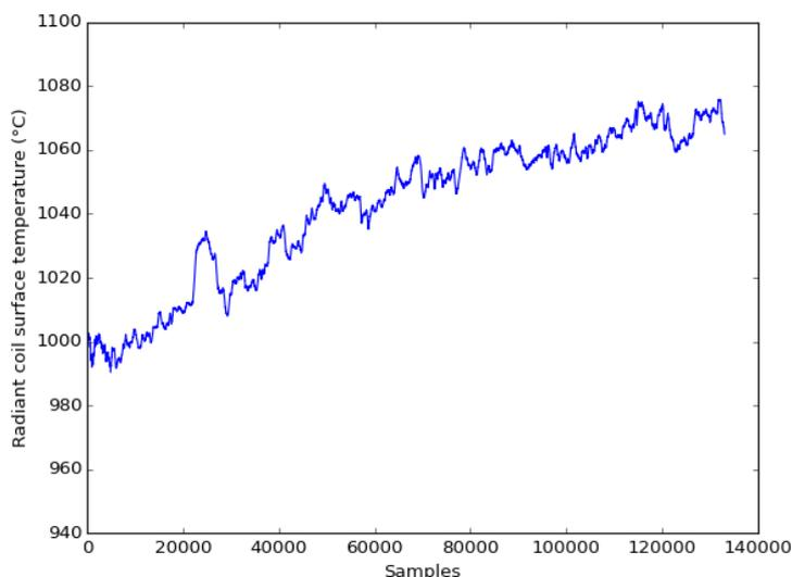
Figure 6: The predicted coil surface temperatures of the first group coils in south side
