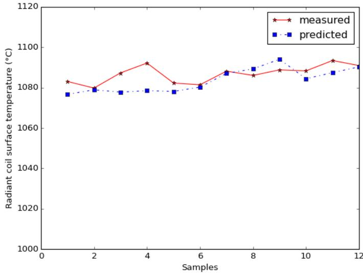
Figure 2: The coil surface temperatures of first group radiant coil in north side
