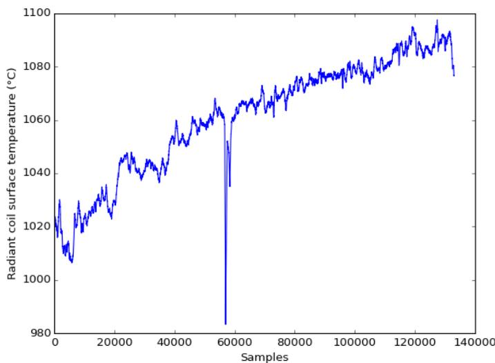
Figure 5: The predicted coil surface temperatures of the first group coils in north side
