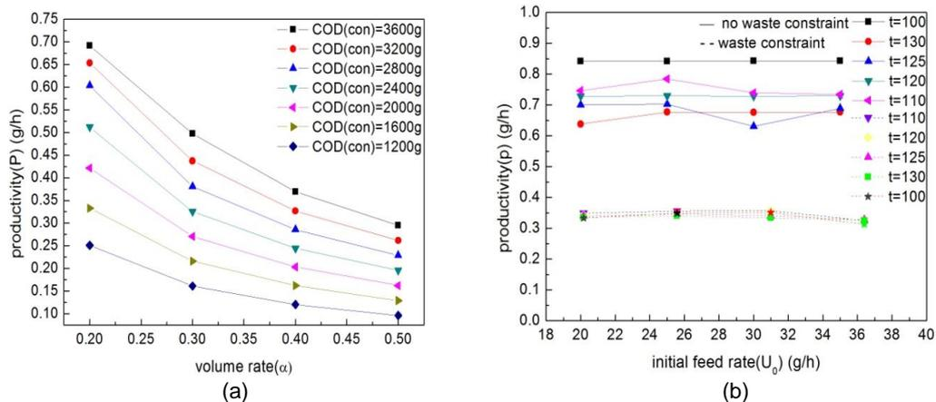
Figure 3 (a): Results under different value of  $\alpha$  and COD(con) when initial feed rate  $U_0=25$ , fermentation time  $t_f = 100$  h; 3(b): The comparison between the two computations with different value of  $U_0$  and  $t_f$
