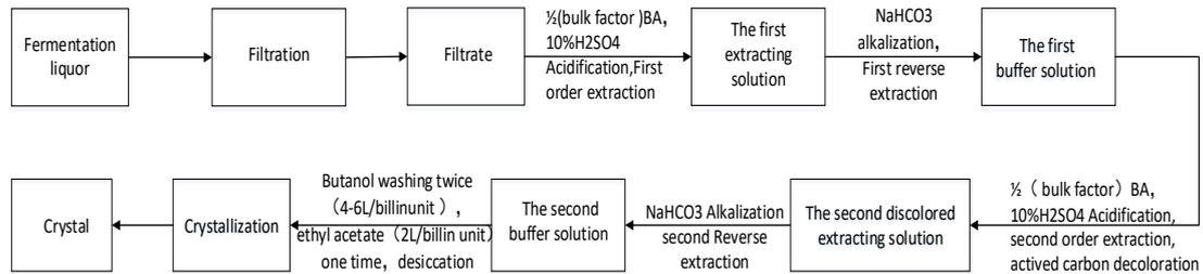
Figure 2: The process of penicillin fermentation flowsheet
