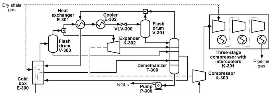
Figure 3: Process flowsheet of NGLs recovery process
