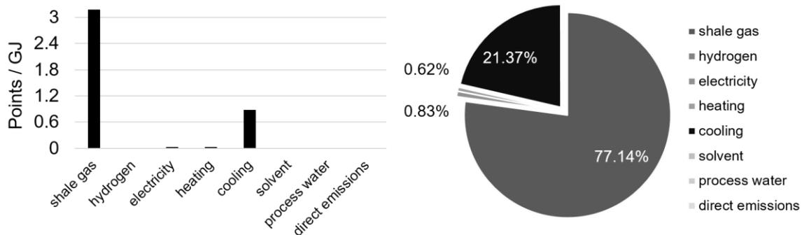
Figure 5: Eco-indicator 99 distribution of the robust process design
