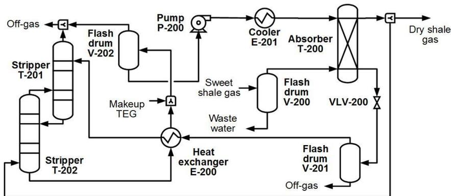
Figure 2: Process flowsheet of dehydration process
