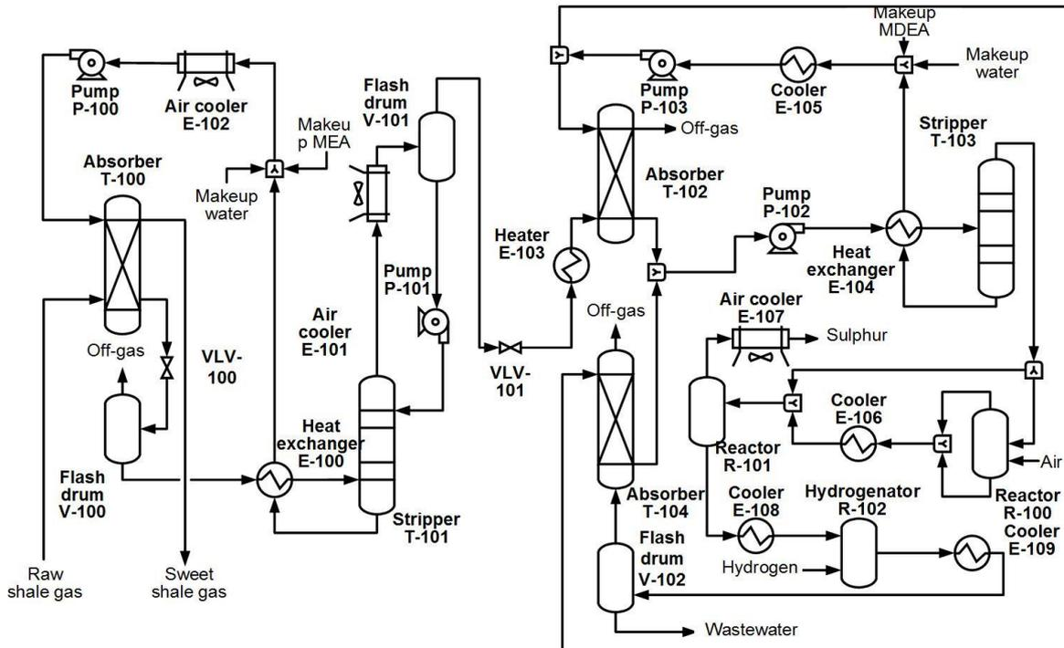
Figure 1: Process flowsheet of acid gas removal process
