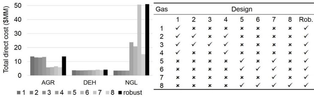
Figure 4: Total direct cost distribution and product qualities of different designs with respect to various gas compositions. Check and cross represent qualified and unqualified product for pipeline gas specifications
