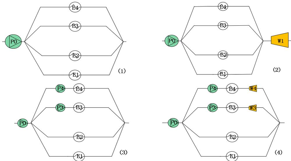
Figure 2: The structures of the fluid machinery network before and after optimization
