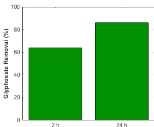
Figure 4. Glyphosate removal with time using  $\text{MnFe}_2\text{O}_4\text{-G}$ .
