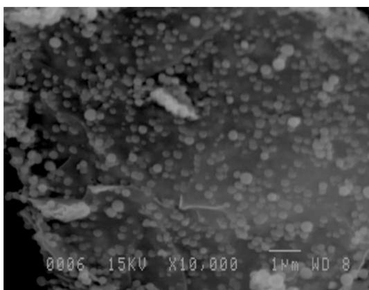
Figure 3. SEM image of  $\text{MnFe}_2\text{O}_4\text{-G}$ .
