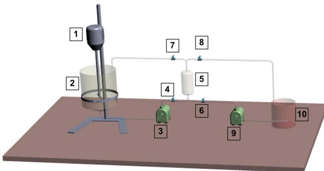
Figure 1. Scheme of pilot batch scale reactor built for this study.
