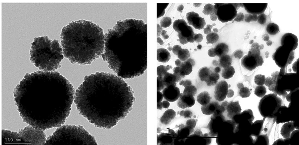
Figure 2. TEM micrograph of  $\text{MnFe}_2\text{O}_4$  (a) and TEM micrograph of  $\text{MnFe}_2\text{O}_4\text{-G}$  (b).
