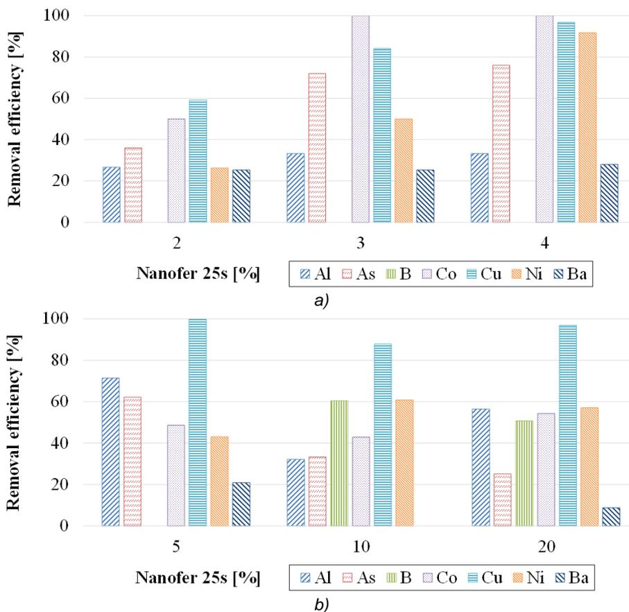
Figure 2: Comparative analysis of the obtained results having used low (2, 3 and 4%) and high (5, 10, 20%) dosage of Nanofer 25s.
