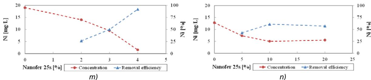
Figure 1: Results of the experimentation having used low (2, 3 and 4%) and high (5, 10, 20%) dosage of Nanofer 25s: (a, b) Al; (c, d) As; (e, f) B; (g, h) Ba; (i, j) Co; (k, l) Cu and (m, n) Ni.
