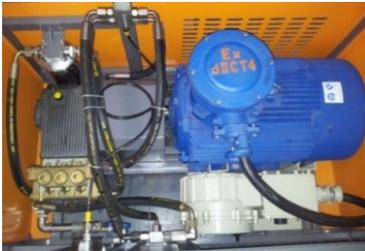
Figure 13: The generation system of portable AWJ high-pressure water
