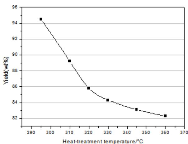
Figure 2: Effect of reaction temperature on the yield of mesophase pitch
