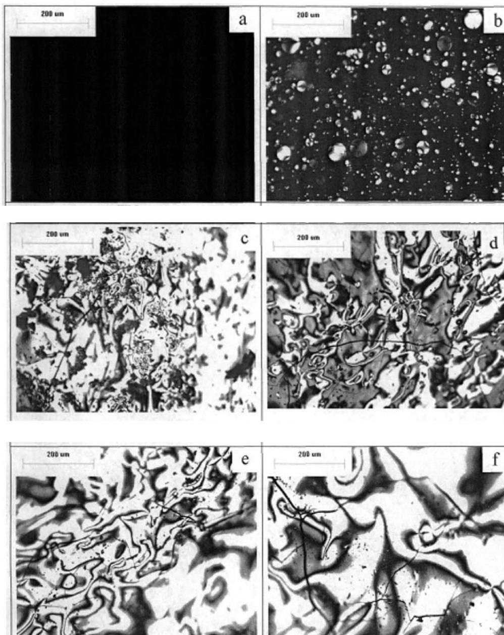
Figure 1: Polarized-light micrographs of mesophase pitches at different treatment temperatures and holding times for coal-tar pitch reaction/ $^{\circ}\text{C}$  (a)  $295^{\circ}\text{C}$ -6h; (b)  $310^{\circ}\text{C}$ -5h; (c)  $320^{\circ}\text{C}$ -5h; (d)  $330^{\circ}\text{C}$ -5h; (e)  $345^{\circ}\text{C}$ -5h; (f)  $360^{\circ}\text{C}$ -2h
