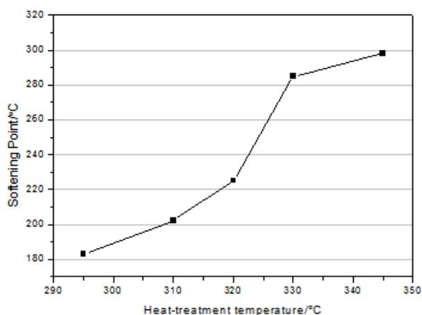
Figure 3: Effect of reaction temperature on the softening point of mesophase pitch
