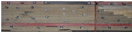
(a) Working face advances to the place 486.5 m away from the slope foot (initial terminal mining line)
