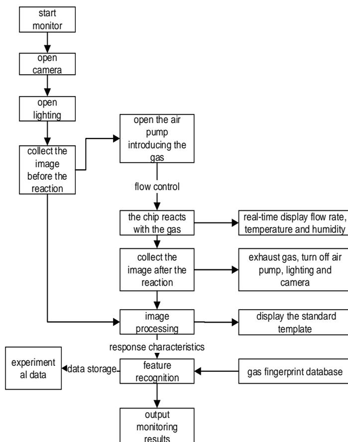
Figure 2: Schematic figure of gas detection system
