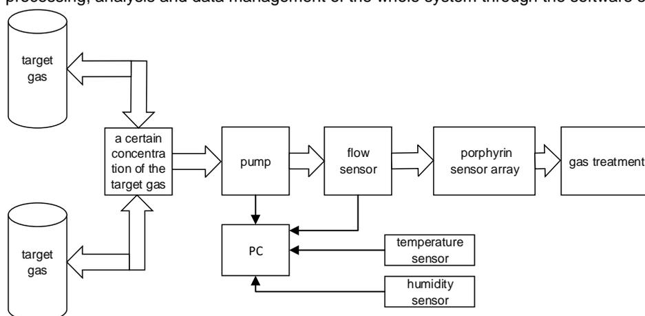
Figure 1: Schematic diagram of porphyrin sensor detection system
