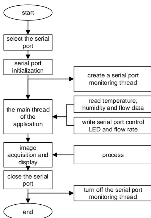
Figure 3: Diagram of serial communication
