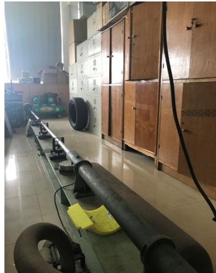
(b) SHPB experimental system
