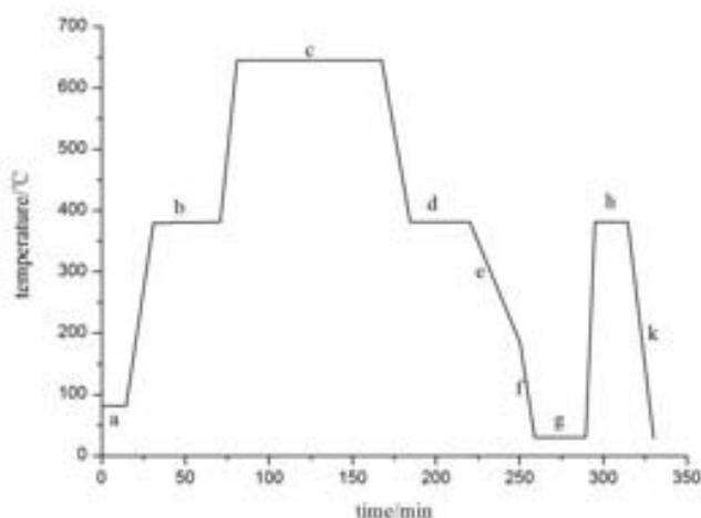
Figure 1: The flow chart of the QPQ process
