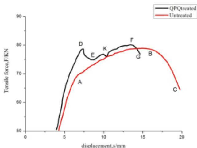
Figure 2: The force and displacement curve of N80 steel treated by QPQ
