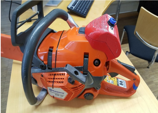
Figure 3: Those pictures represent the innovative developed device. It is a dedicated and customized device, which perform synchronized (10 Hz) acceleration and GNSS detections.
