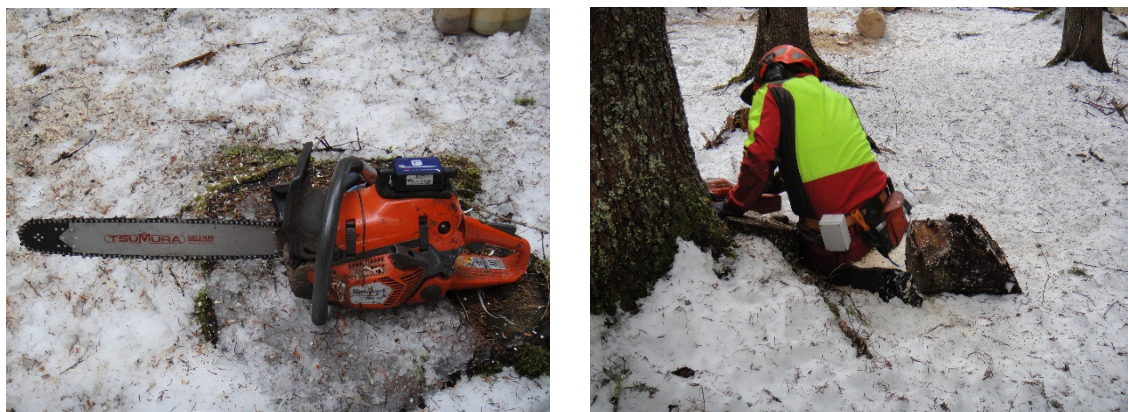
Figure 1: The left figure shows the chainsaw equipped with accelerometer, while the right shows the operator during the felling procedure. In the white box, fixed at the belt, is placed the GPS.
