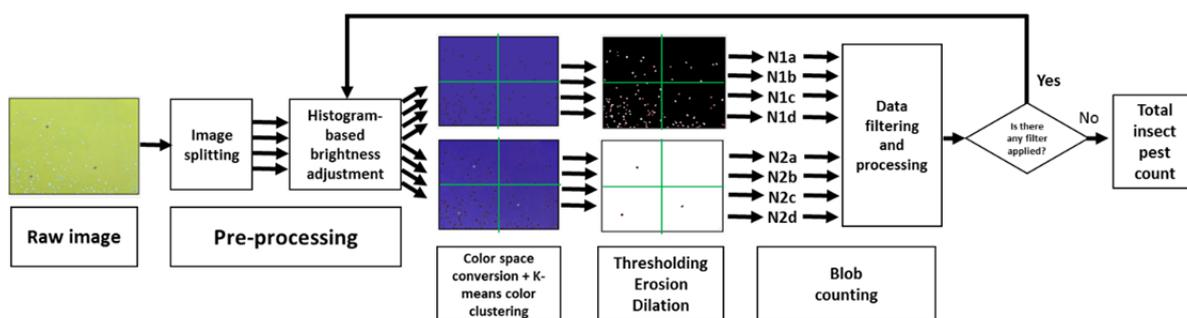
Figure 4: Insect pest counting image and data processing algorithm flowchart
