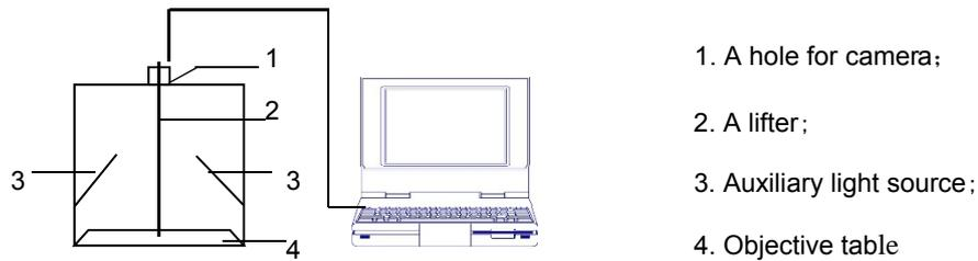
Figure 1 Experiment box for taking pictures
