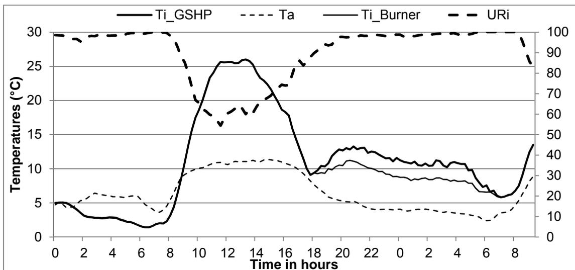
Figure 5: Ambient air temperature, internal air temperatures and humidity of the two twin greenhouses.
