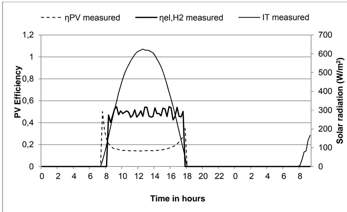
Figure 3: Solar radiation, PV and electrolyzer efficiency of the stand-alone hydrogen plant.
