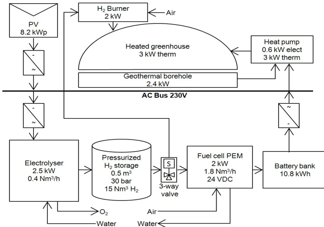
Figure 1: PV, GSHP and hydrogen heat generator in a stand-alone system for greenhouse heating.
