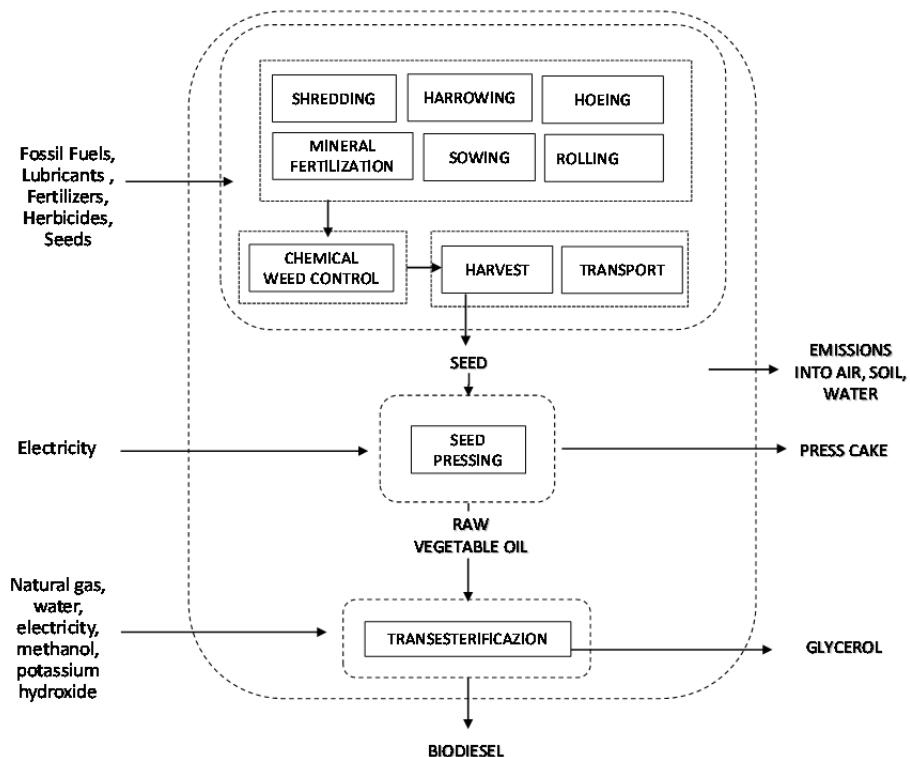
Figure 1: System boundary of the biodiesel production process
