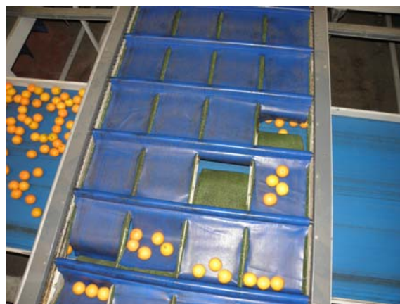
Figure 3: The innovative line feeding system (bin emptying). Figure 4: The innovative strip conveyor.
