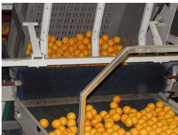
Figure 3: The innovative line feeding system (bin emptying). Figure 4: The innovative strip conveyor.
