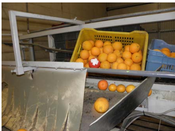
Figure 1: The conventional line feeding system (box emptying).
