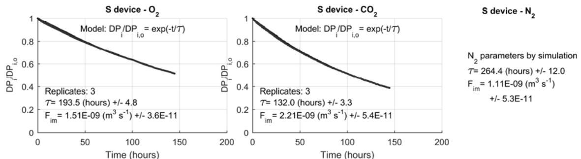
Figure 1: Operative characteristics of smart device used for trials.  $F_{im}$  represents the diffusion coefficient measured for O<sub>2</sub>, CO<sub>2</sub> and N<sub>2</sub>.  $DP$  represents the differential pressure across the smart device,  $DP_o$  represents the initial differential pressure.  $\tau$  is the smart device measured time constant that is related to  $F_{im}$ .
