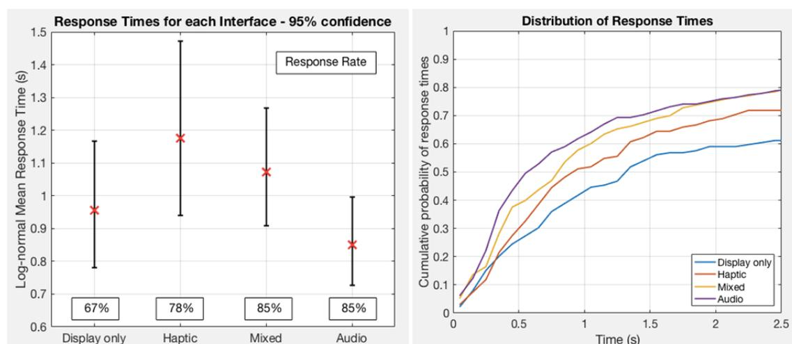
Figure 5. The mean response times have a wide confidence interval, but the cumulative probability functions show that the auditory alert produced the largest number of effective responses in shorter time periods.
