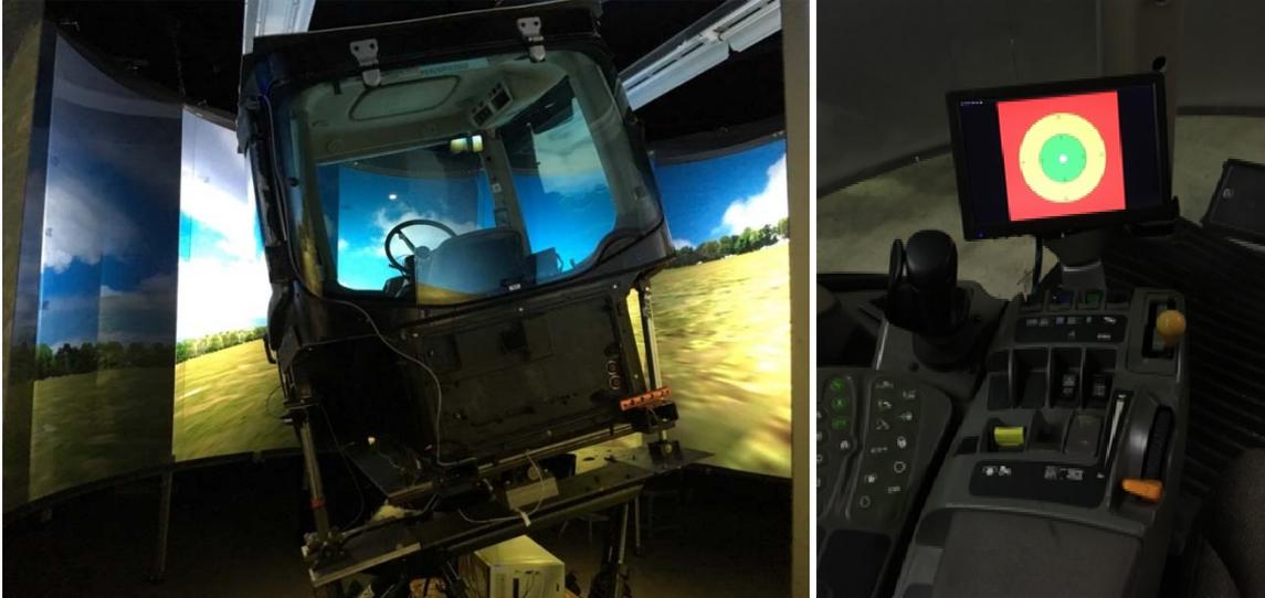
Figure 1. The tractor driving simulator has a digital bubble-level display on the armrest instrument panel.
