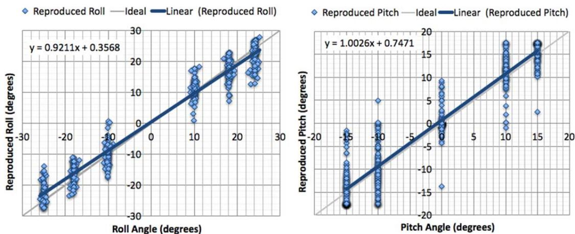
Figure 3. Regressions show that roll was consistently under-produced, and therefore overestimated by a factor of 8%. Pitch angles however, on average, was reproduced accurately.
