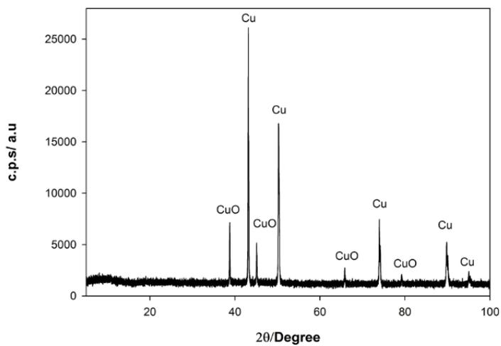
Figure 2: Diffraction pattern of the copper deposit
