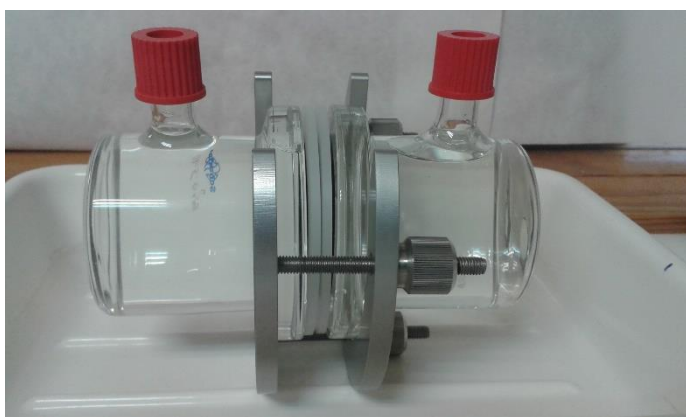
Figure 1: Image of the cell where the SILMs tests were carried out
