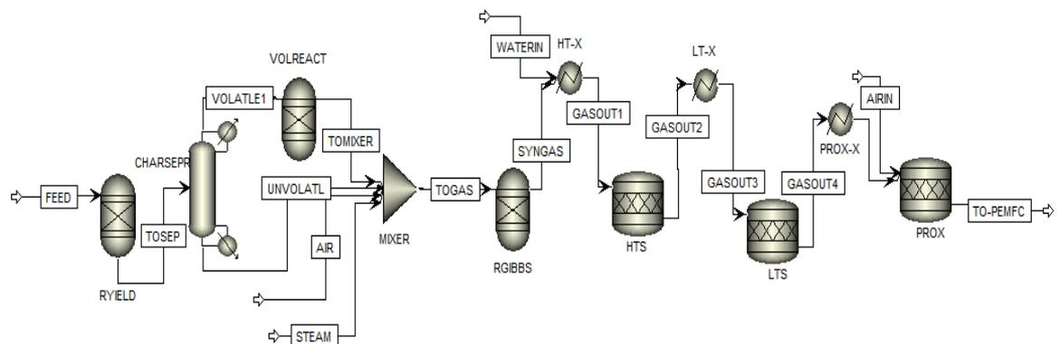
Figure 2: Fluidised bed gasification process with hydrogen purification flowsheet
