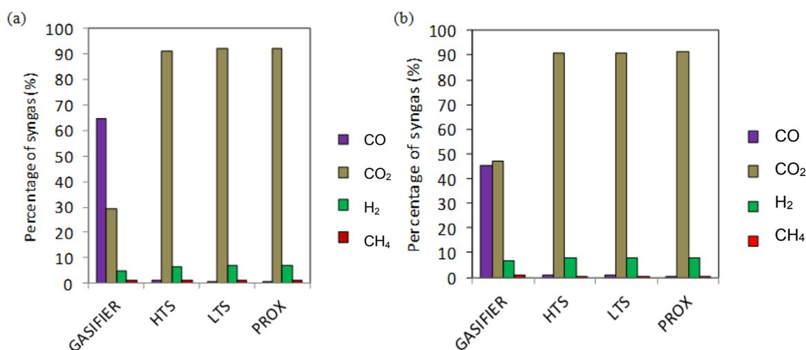
Figure 3: Product gas percentages at the outlets of the gasifier, HTS reactor, LTS reactor and PROX reactor from (a) fixed bed, (b) fluidised bed
