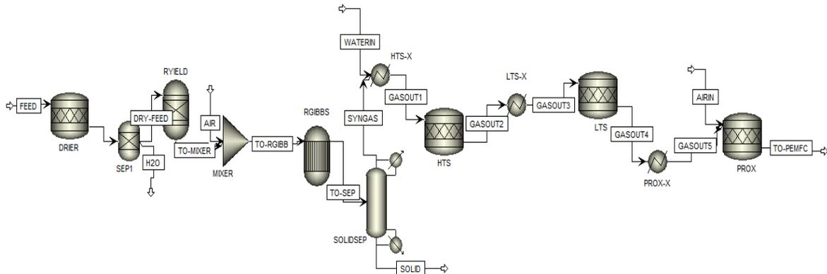
Figure 1: Fixed bed gasification with hydrogen purification flowsheet
