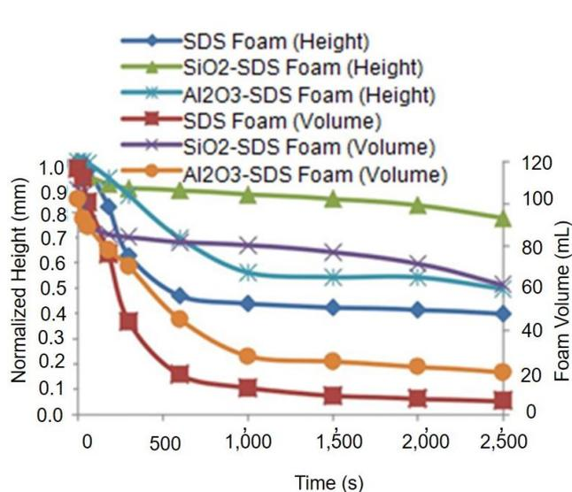
Figure 2: Normalised foam height and foam volume of SDS and nanoparticles-SDS foams with respect to time
