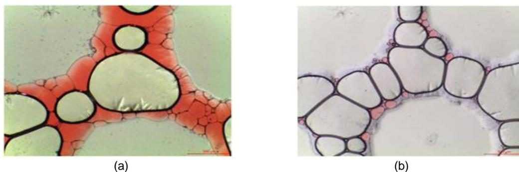
Figure 4: Foam flow process in presence of paraffin oil in etched glass micromodel for (a) SDS-stabilised foam and (b) SiO<sub>2</sub>-SDS stabilised foam
