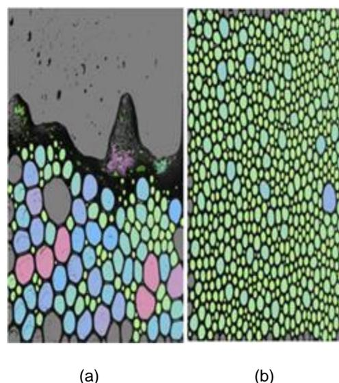
Figure 3: Bubble size distribution of (a) SDS-stabilised foam and (b)  $\text{SiO}_2$ -SDS stabilised foam after 60 min
