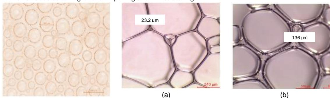
Figure 5: Foam image of Al<sub>2</sub>O<sub>3</sub>-SDS foam showing aggregation
