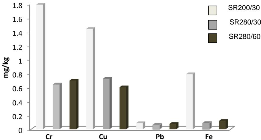
Figure 4: The total content of Cr, Cu, Fe and Pb in liquid phase after SCW treatment
