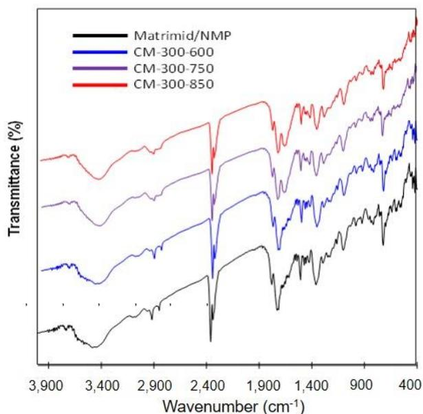
Figure 1: FTIR analysis of Matrimid-based carbon membranes prepared at different carbonisation temperature
