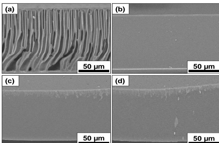
Figure 2: SEM images of the cross-sections for Matrimid/NMP-based (a) Polymeric membrane, (b) CM-600, (c) CM-750 and (d) CM-850
