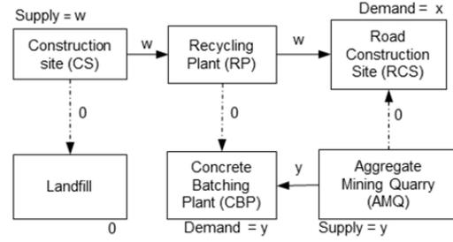
Figure 2: System boundary for scenario 1, BaU (landfilling) Figure 3: System boundary for scenario 2 where CW is recycled as road base material
