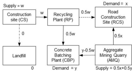
Figure 4: System boundary for scenario 3 where CW is recycled as road base material and reused to produces RAC.
