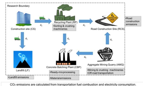
Figure 1: System boundary of CW life cycle assessment.
