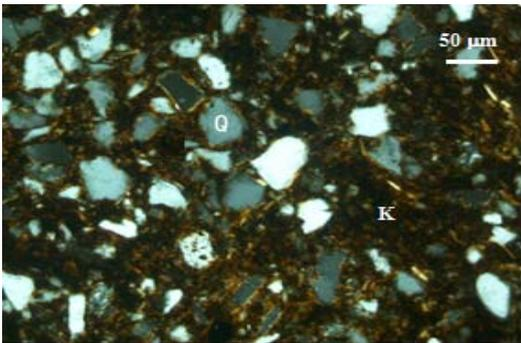
Figure 4: Fe- impregnated kaolinite (K) distributed along the edge of quartz (Q) Cross-polarized light
