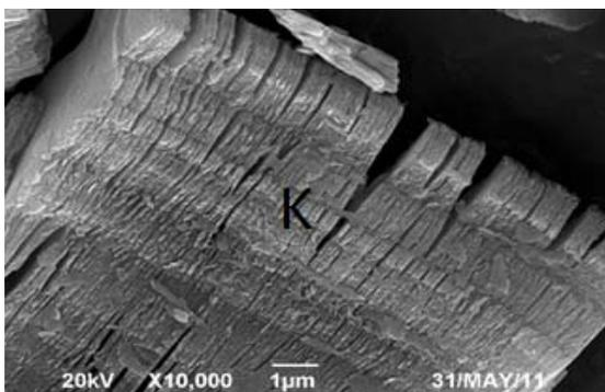
Figure 2: Tiny schistose kaolinite (K) aggregated in book-like form Secondary Electron Image
