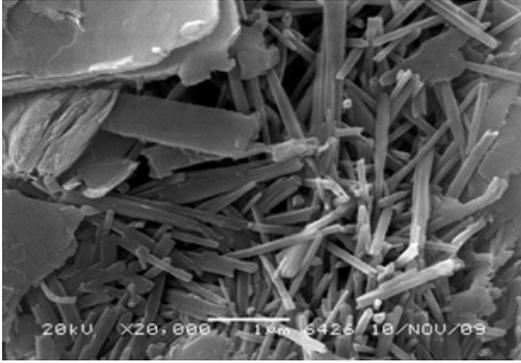
Figure 3: Kaolinite in micro-crystalline tube form Secondary Electron Image
