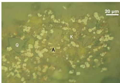
Figure 7: Fine grain-sized anatase (A) disseminated distribution in kaolinite (K), Q-quartz, reflective light
