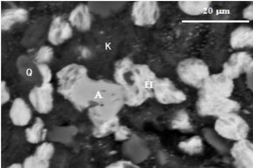
Figure 5: Hematite (H) scatteredly distributed in kaolinite (K), A-anatase, Q-quartz BSE
