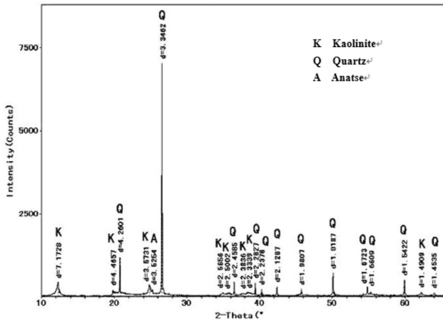
Figure 1: X-ray diffraction pattern of the ores
