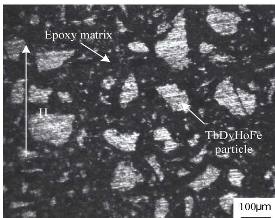
Figure 1: Optical micrograph of the  $\text{Tb}_{0.25}\text{Dy}_{0.45}\text{Ho}_{0.31}\text{Fe}_{1.9}/\text{epoxy}$  composites
