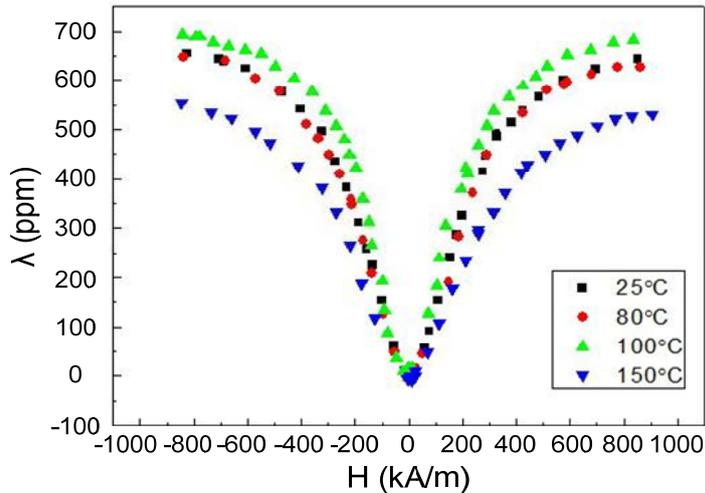
Figure 5: Magnetostriction curves after annealing at 25, 80, 100 and 150 °C ( $x=0.31$ )
