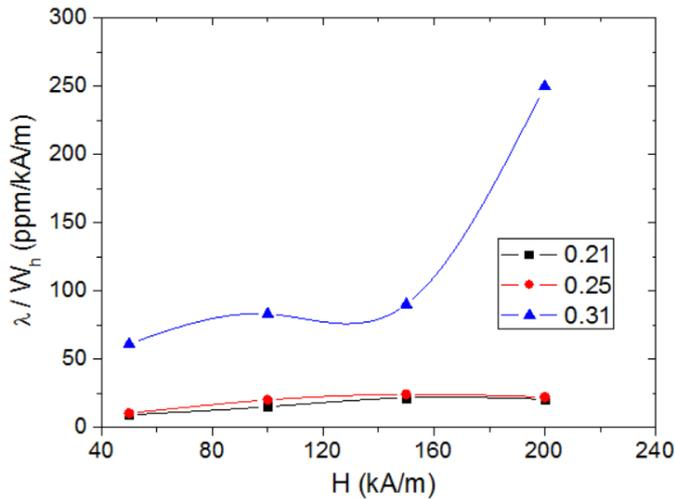
Figure 4: The ratio of magnetostriction to hysteresis width ( $\lambda/W_h$ ) of  $(Tb_{0.15}Ho_{0.85}Fe_{1.9})_x+(Tb_{0.3}Dy_{0.7}Fe_{1.9})_{1-x}$ /epoxy composites with  $x=0.21, 0.25$  and  $0.31$
