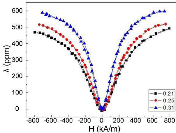
Figure 2: The  $\lambda$ - $H$  curves of  $(Tb_{0.15}Ho_{0.85}Fe_{1.9})_x+(Tb_{0.3}Dy_{0.7}Fe_{1.9})_{1-x}$ /epoxy composites with  $x=0.21$ ,  $0.25$  and  $0.31$
