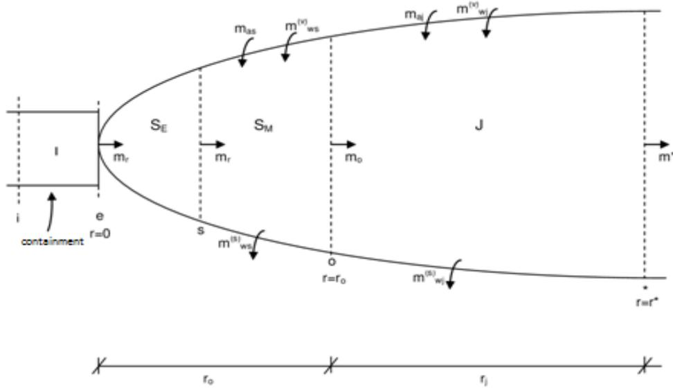
Figure 1: Schematization of the horizontal jet physical model according to three ideal region evolution.
