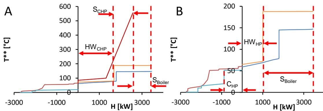
Figure 2: Total Site Profiles for wet processes of the whey powder process. System A: piston-engine CHP integration. System B: Heat Pump integration.
