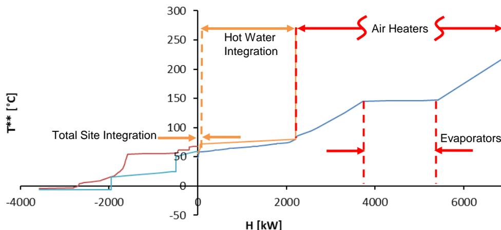
Figure 1: Total Site Profiles for the whey separation and drying process.
