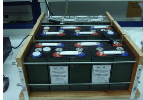
Figure 4: Lithium-Ion Battery stack of the hybrid system
