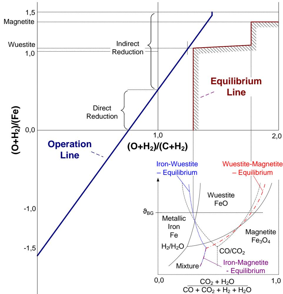
Figure 2: Example of a Rist operating diagram
