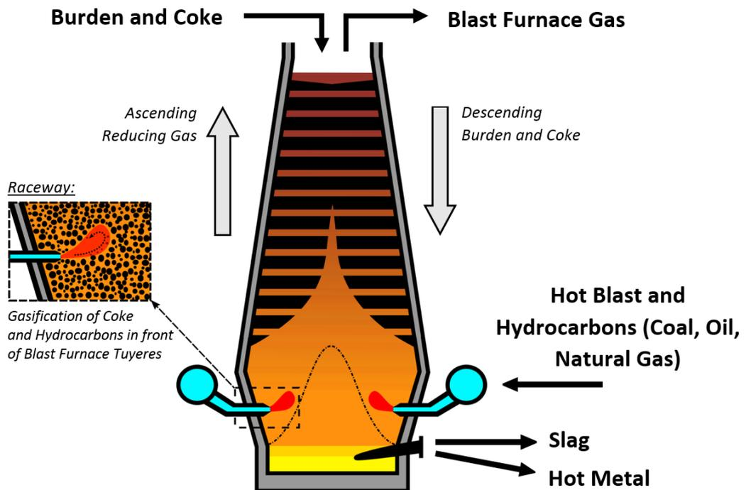
Figure 1: Blast furnace process overview
