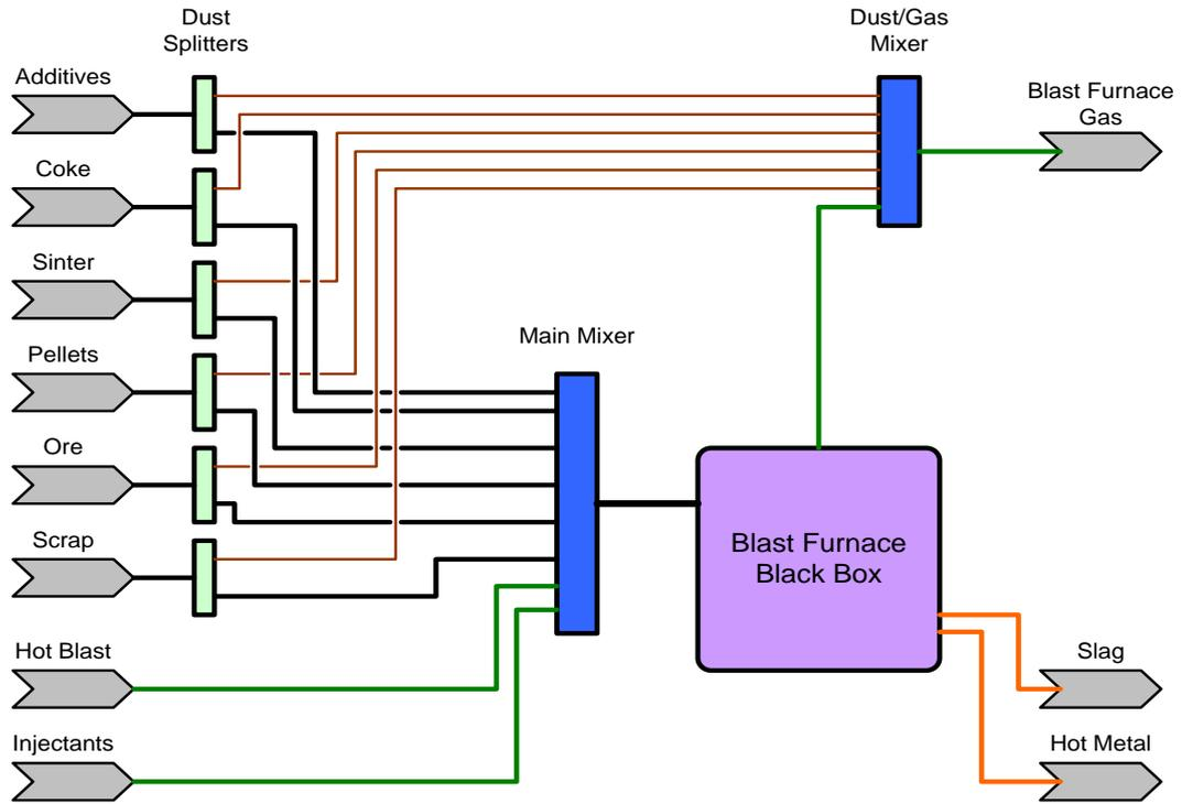
Figure 3: Main sub topology layer of the blast furnace model
