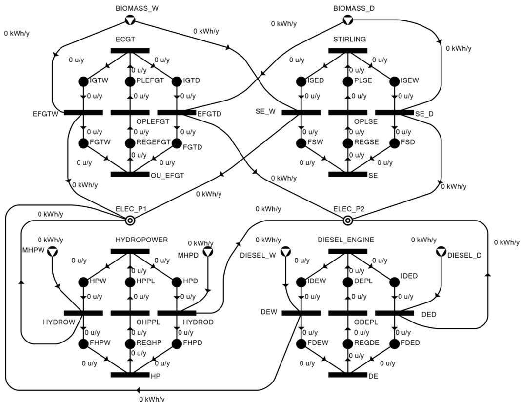
Figure 2: Maximal structure of electricity generation network for case study
