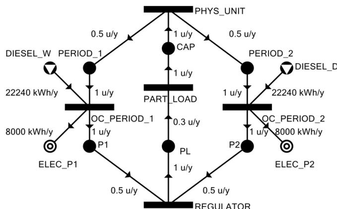
Figure 1. Multi-period P-graph representation for Diesel Engine
