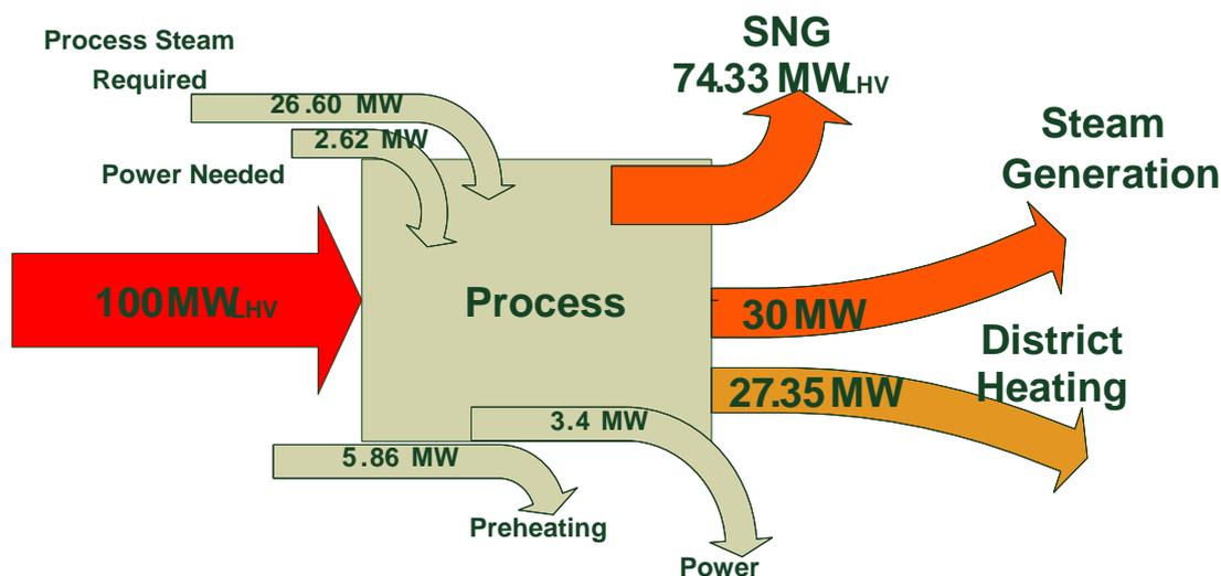
Figure 2: Energy balance of the system
