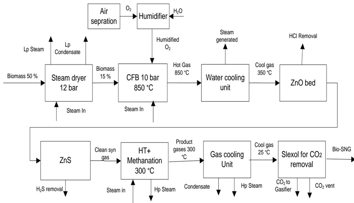
Figure 1: Developed process flow of SNG Production from Biomass gasification
