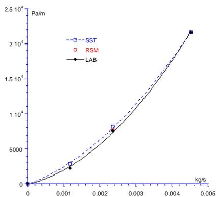
Figure 3: Static pressure drop per unit HEX length (from inlet to outlet) comparison
