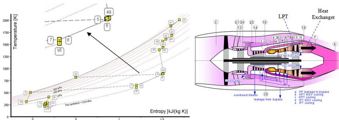
Figure 9: The MTU intercooled recuperative cycle (average cruise conditions) in Gas turb11
