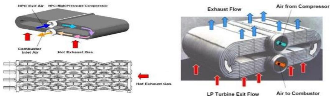
Figure 1: The MTU-heat exchanger (4/3/4 core)
