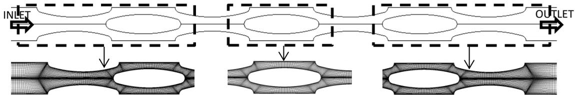
Figure 2: The 2D CFD model of the HEX flow path
