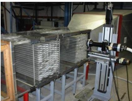
Figure 5: HEX core 10:1 experimental setup
