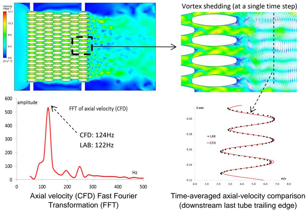
Figure 7: CFD results of the 2D model and comparison with experimental measurements
