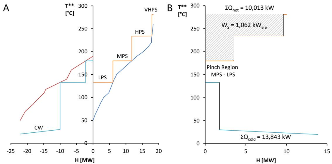
Figure 3: Conventional TSP (A) and SUGCC (B).
