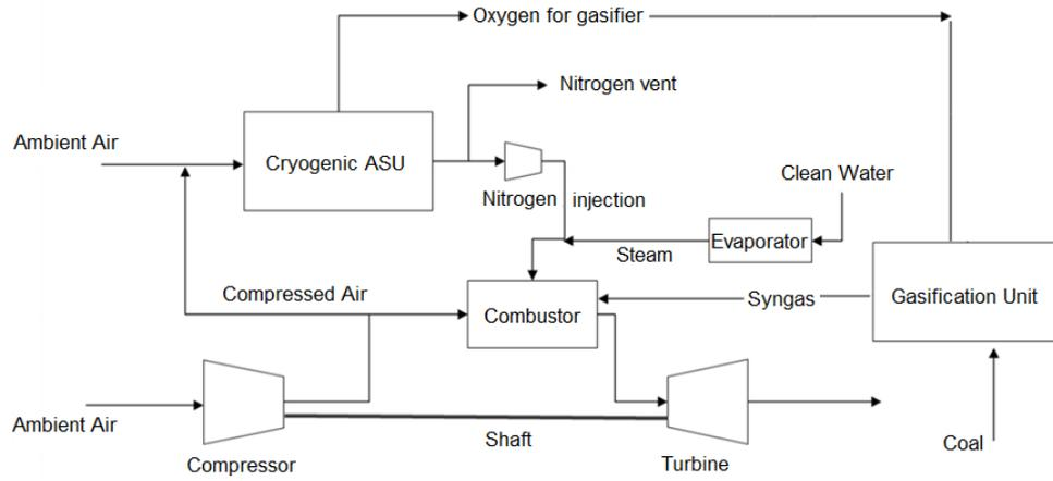
Figure 1: Schematic diagram of the IGCC process.
