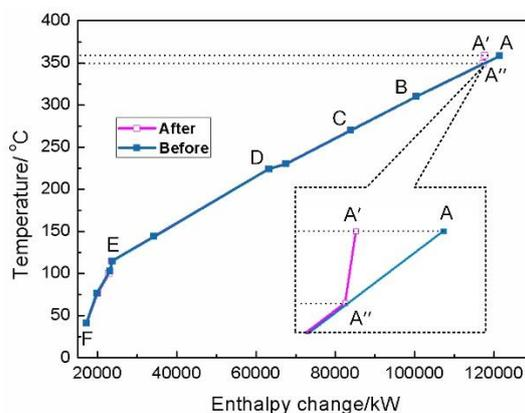
Figure 3: The change of Sink Composite Curve
