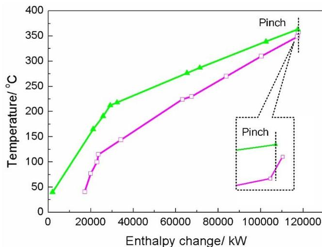
Figure 6: The Composite Curve plotted by the original Pinch Method
