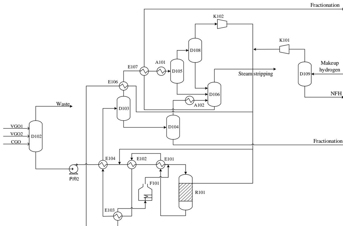
Figure 1: Process flowsheet of VGO hydrotreating process
