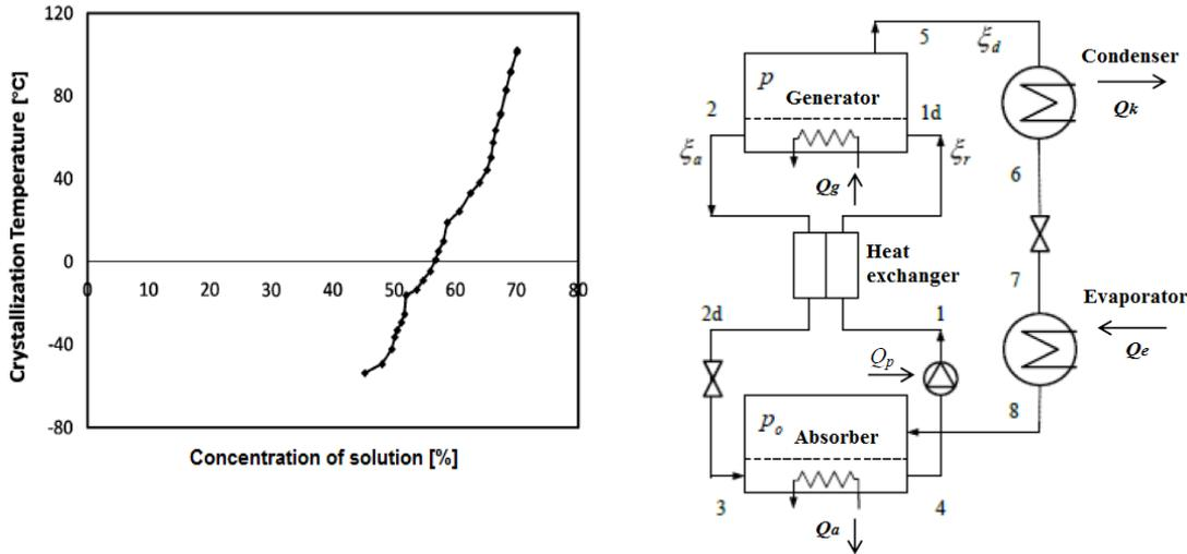
Figure 1: Solubility of pure LiBr in water (Boryta, 1970) Figure 2: Schematic of an absorption cooling device
