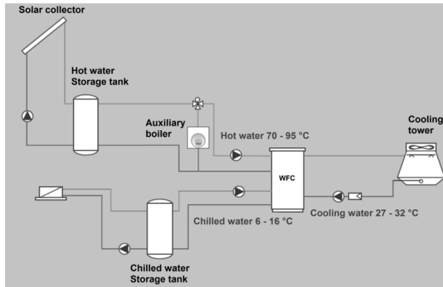
Figure 6: Process flow diagram of solar cooling system in Dubrovnik
