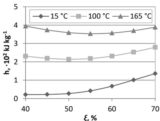
Figure 4: Specific enthalpy of LiBr/H<sub>2</sub>O solution
