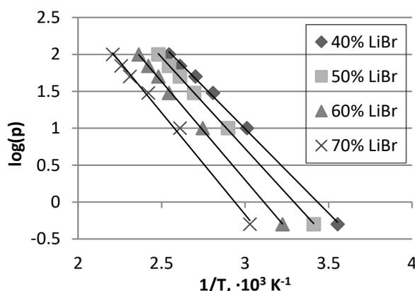
Figure 3: Pressure dependence on temperature for LiBr/H<sub>2</sub>O
