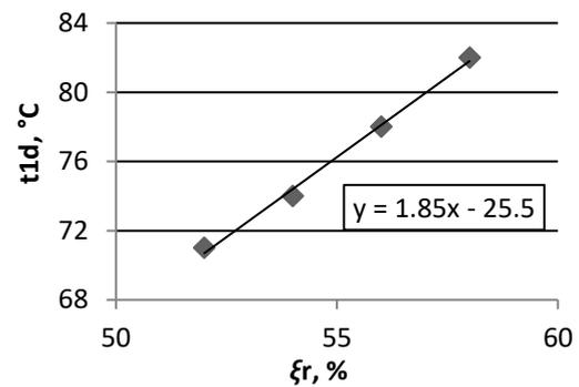
Figure 11: Temperature at the generator input depending on the concentration of weak solution
