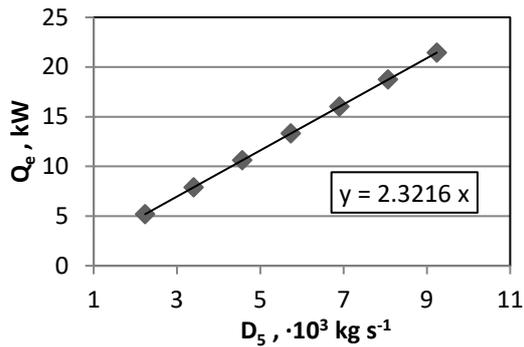
Figure 10: Cooling capacity depending on the mass flow rate of evaporated pure water
