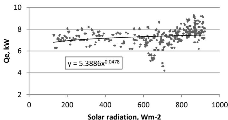
Figure 9: Measured cooling capacity depending on solar radiation on the 21<sup>st</sup> July 2015 from 9 am to 7 pm
