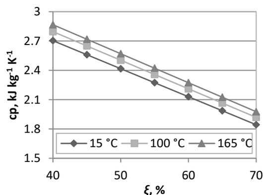
Figure 5: Specific heat capacity of LiBr/H<sub>2</sub>O solution
