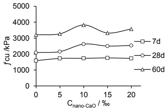
Figure 1: Relationship between  $f_{cu}$  (kPa) and nano-CaO content (‰)
