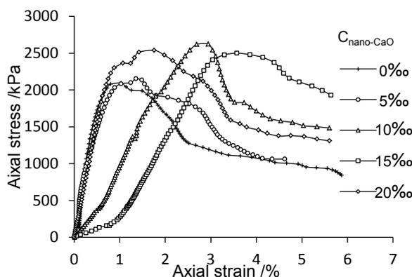
Figure 3: Stress-strain curves after 28 d of curing
