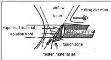
Figure 1: Laser machining process
