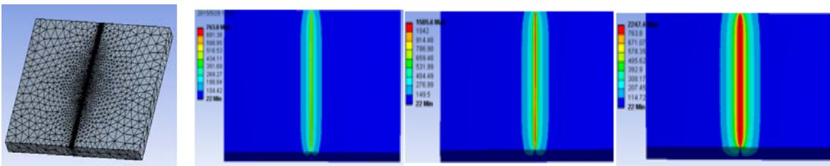
Figure 6: Mesh model Figure 7: The temperature field distribution of target under different laser power density
