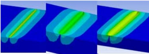
Figure 8: The ablation crater morphology of target under different power density
