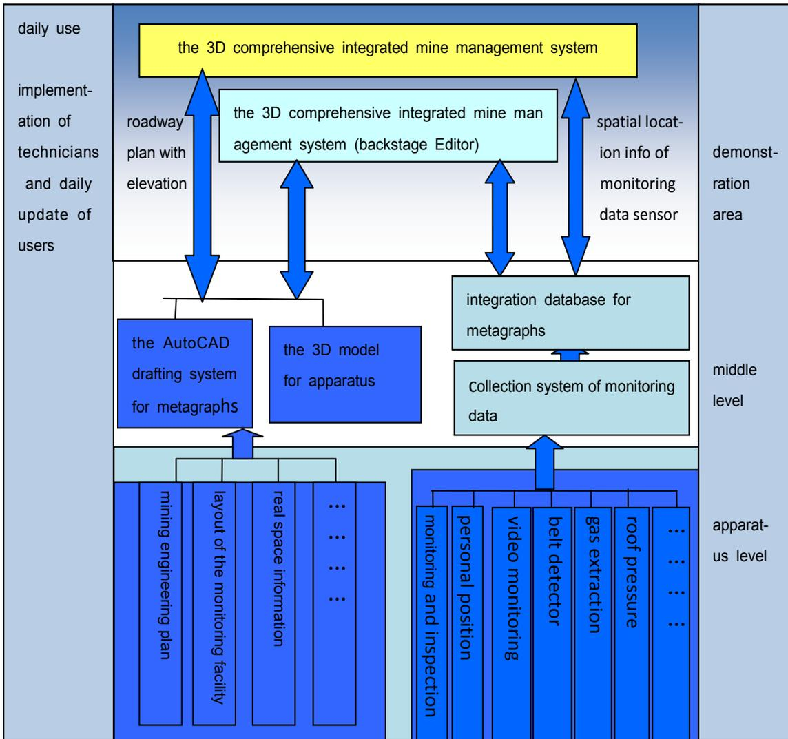
Figure 1: Framework design and features of the system
