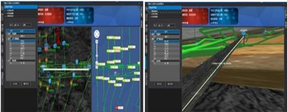
Figure 4: Personnel positioning and historical track playback of Baobao mine 3D Integrated Management System
