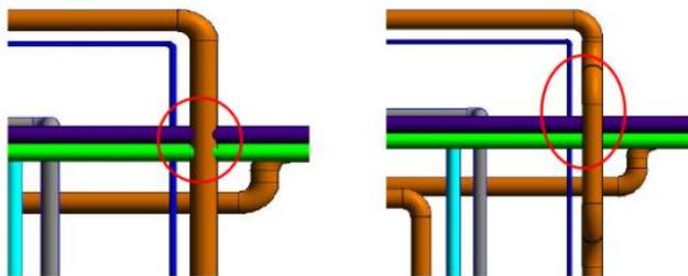
Figure 2: Pipeline collision schematic diagram
