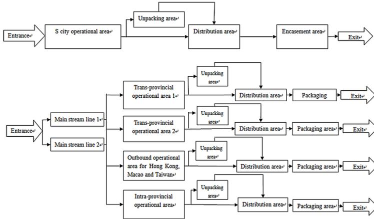
Figure 2: Flow block diagram of simulation model for distribution center.
