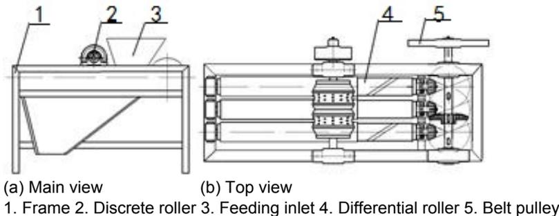
Figure 1: Discrete test-bed of corn ear
