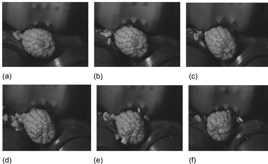
Figure 4: Working process of the discrete roller with high-speed photography
