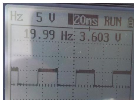
Figure 12: Frequency output map of motor at low speed rotational
