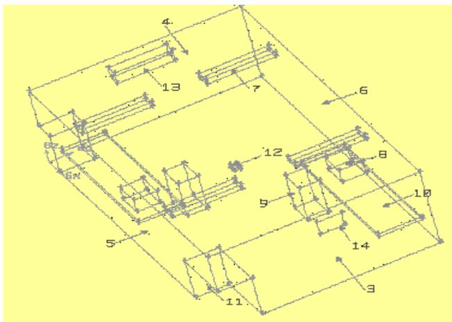
Figure 2: The mixed ventilation air conditioning system model in the office (Side to side back to type)
